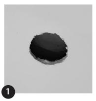
Drill hole into mounting surface (Ø35mm/1.38").
